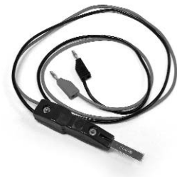
Fig. 3.7: Current Test Plug
