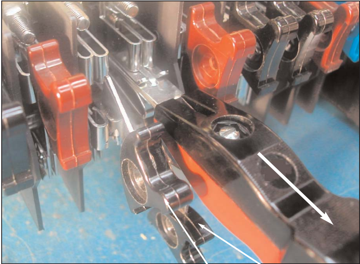
Fig. 3.18: Remove Test Plug from Shunt Jack
